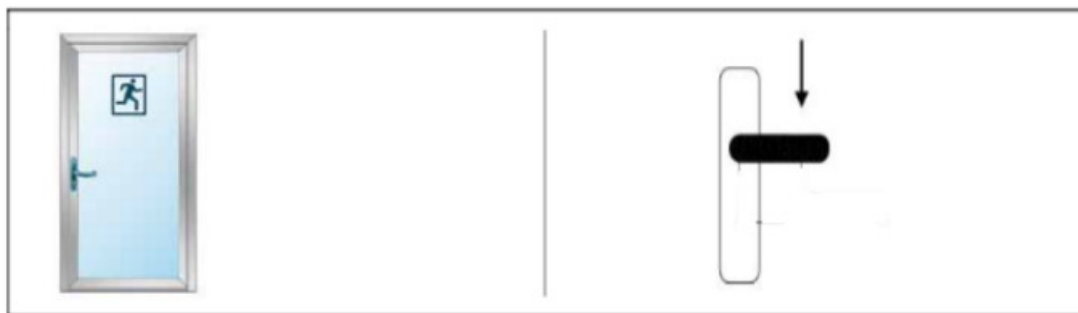
Picture 32. How to open a panic door with a push handle according to EN 179
